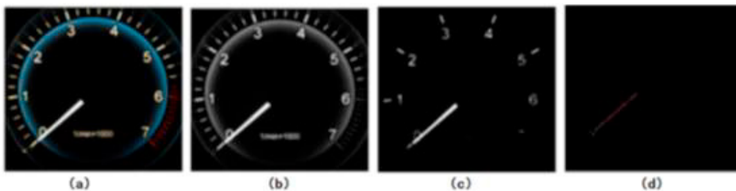
Fig.3. (a)Engine tachometer image; (b) Gray image; (c)Binary image; (d) Hough transform the result
